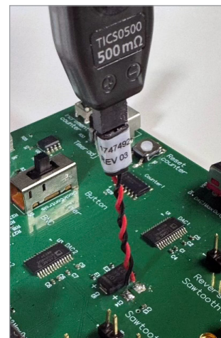
Figure 8. Using a probe-based wideband shunt connected via twisted pair.
